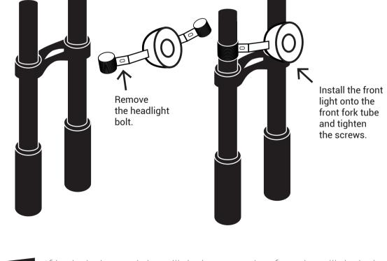
If included, attach headlight by removing front headlight bolts and positioning headlight before loosely screwing bolts back in place. Finally, adjust the headlight to the desired position
