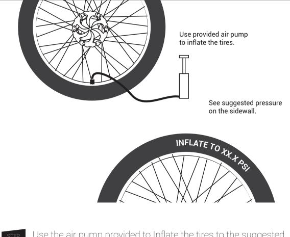
Use the air pump provided to Inflate the tires to the suggested pressure indicated in the sidewall of the tire.
