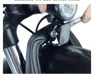
Connect the wiring to the headlights
