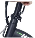
Press the key towards the keyhole and turn the key to the "PUSH" button to remove the battery
