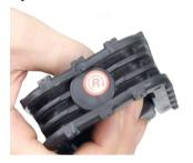
Push the rear seat cushion backward to separate the rear seat cushion from the hole to remove the rear seat cushion
