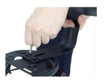
Insert the seat tube, adjust it to a proper height, and lock the quick release handle in the direction
